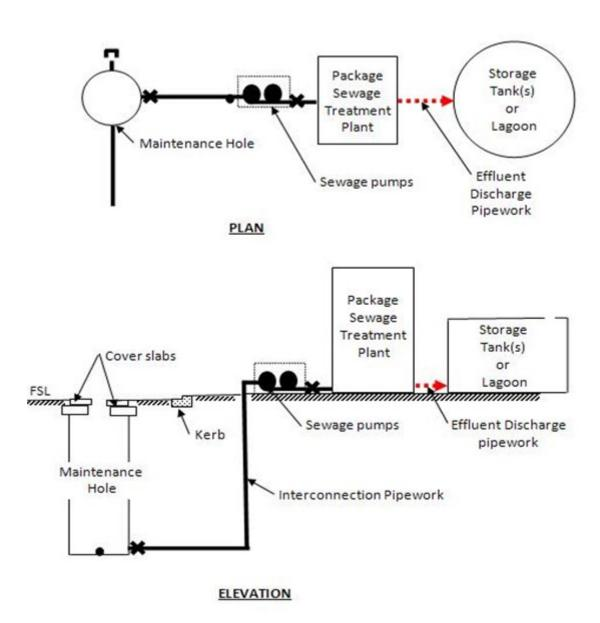
Figure 3 – Temporary on-site treatment and disposal
