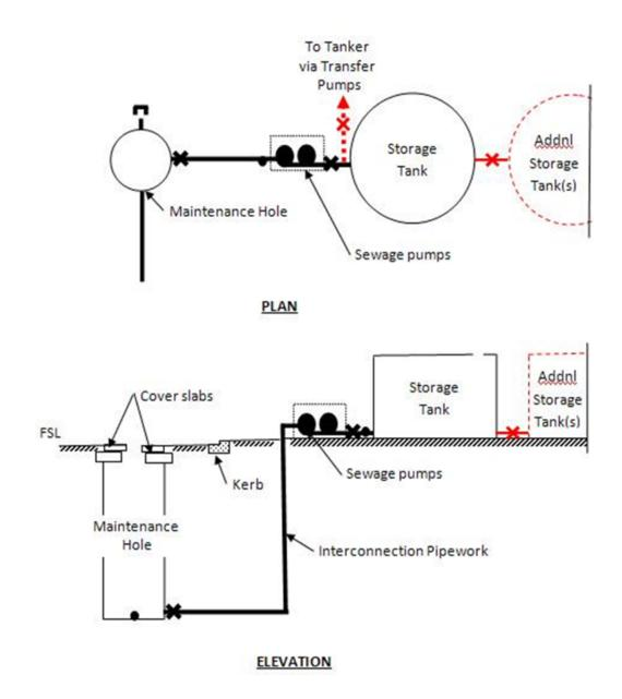
Figure 2 – Temporary on-site storage with tankering
