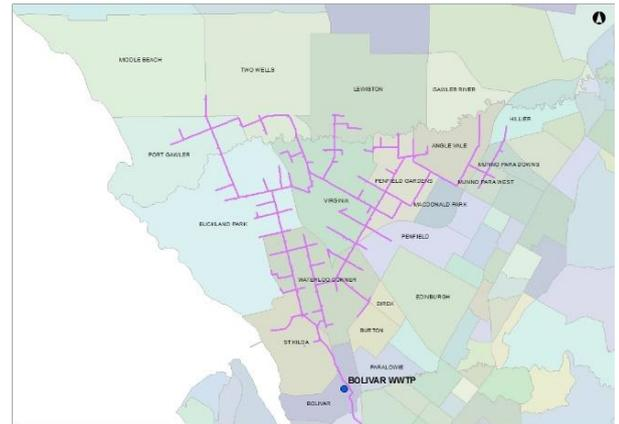
As a comparison, the existing Virginia Pipeline Scheme (pictured right) currently delivers around 17 GL of recycled water from the Bolivar Wastewater Treatment Plant for irrigation use by around 350 irrigators in the Northern Adelaide Plains.
