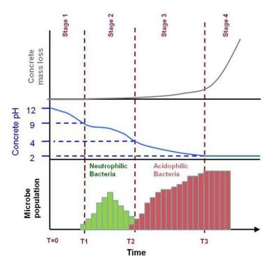
Figure 5-3 Progression of microbial corrosion of sewer pipe
