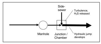
Figure 7-3 Sewer Design to Avoid Hydraulic Jumps
