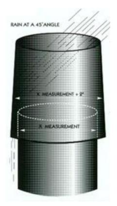
Figure 12-1 Collar-type rain guard for a stack
