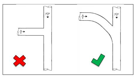
Figure 7-5 Streamlining branch sewer connections on trunk mains
