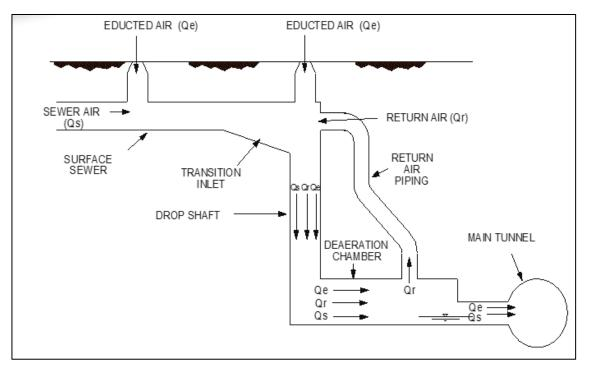
Figure 6-4 Typical Vortex Dropper with Air Return
