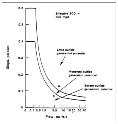
Figure 8-3 Guide for Estimate Sulphide Generation Potential [9]
